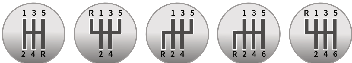
These are some of the most common gear stick layouts
